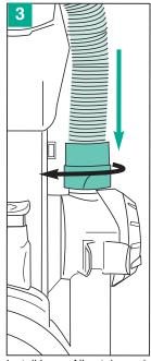
Install hose: Align tabs and push down; twist clockwise to lock.
